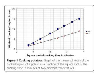
Figure 1 shows the results of one such carefully controlled set of experiments. The data in the figure illustrate that the heat flowing into a potato in a constant temperature bath does indeed follow the expectations of thermal diffusion – the width of the cooked region increases as the square root of the cooking time; and the rate at which this width increases depends on the temperature difference between the potato before immersion and the temperature of the heat bath.
